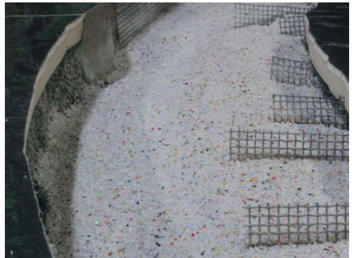
Galvanized wire mesh dikes in HSR model.
